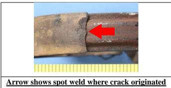
Arrow shows spot weld where crack originated leading to total failure of the outer band and separation of the tailpipe coupling.
