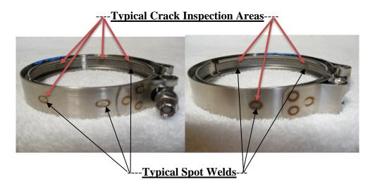
If any of the above conditions are found, the v-band coupling is considered unairworthy and should be removed and replaced before further flight with a new, zero time in service (TIS), FAA-approved coupling according to the instructions and procedures found in the airframe or engine ICA's, as applicable. All v-band couplings removed from service should be permanently destroyed and not used on any other aircraft or aircraft application.
