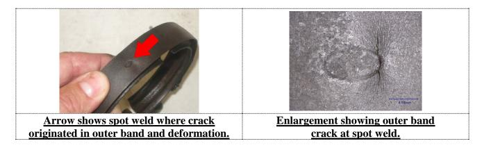
Reference: turbocharger exhaust inlet
